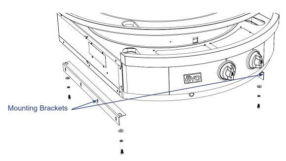
**STEP 6:** Remove two (2) mounting brackets with 7/16" Open End Box Wrench installed on Evo Affinity 30G Cooktop.
