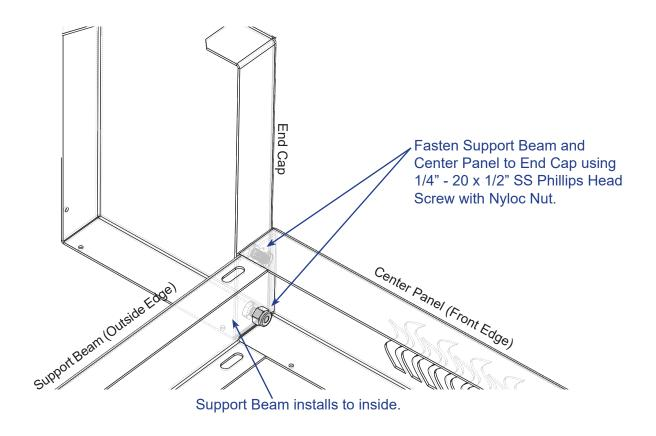
**STEP 2:** Locate Support Beam and Center Panel as shown, and fasten in place with two (2) 1/4" - 20 x 1/2" SS Phillips Head Screws with Nyloc Nuts.
